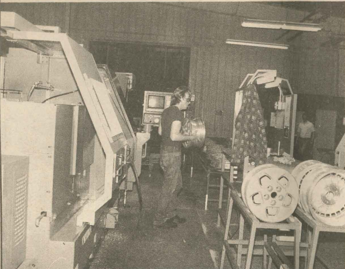
CNC lathes (Computerized Numerical Control) ensure uniformity of production and worker safety. The wheels arrive at the lathe, from the foundry line, and are turned inside and outside for quality finish and inspection. The machines all have state of the art safety features. The Chiron has a multi-position spindle and can drill at multiple positions. The machine is capable of eight tool changes at less than one second per tool change. All are done by air. It is regarded as one of the fastest tools in North America. Machine shop manager Ben Crabbe said safety is ensured as the operator views computerized screen controls. Photo by Jack Britt
